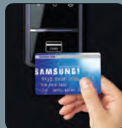
Smart Card RF card or other smart card (Mifare can be used for the access)
